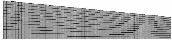
Figure 5: Skewed conforming mesh
