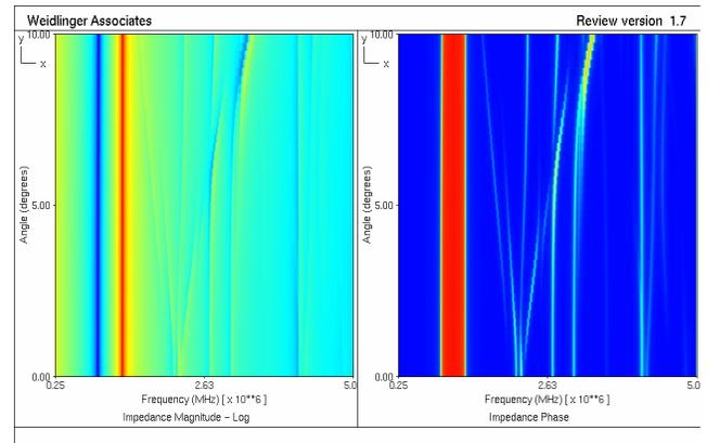
Figure 10: Impedance response for 0.75mm wide trapezoid ( $|Z|$  - left,  $\angle Z$  - right)
