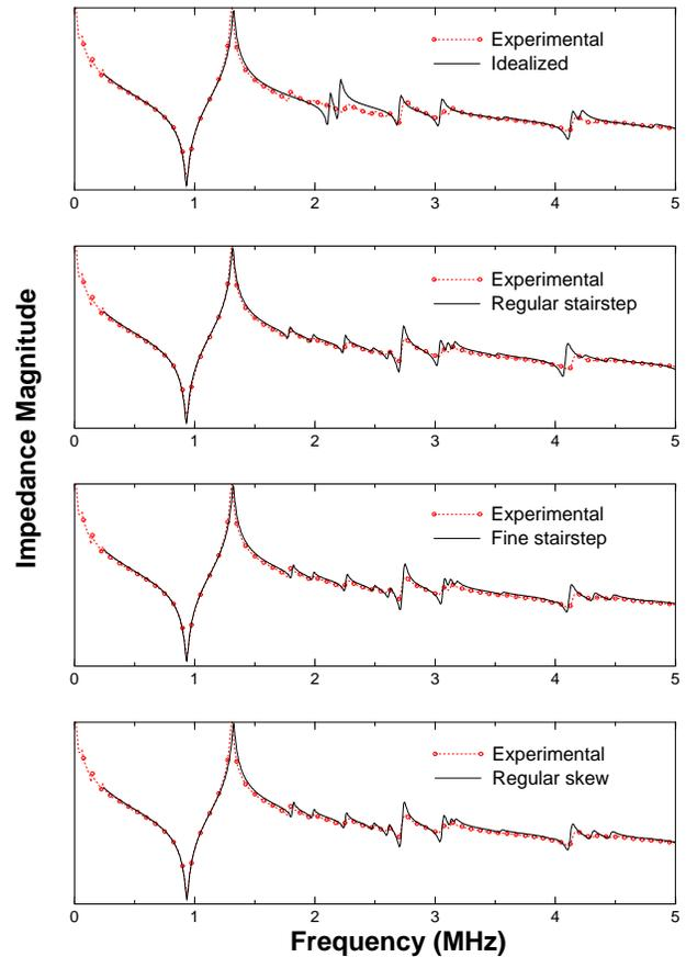
**Figure 7: Impedance response for 0.75mm wide trapezoid**
