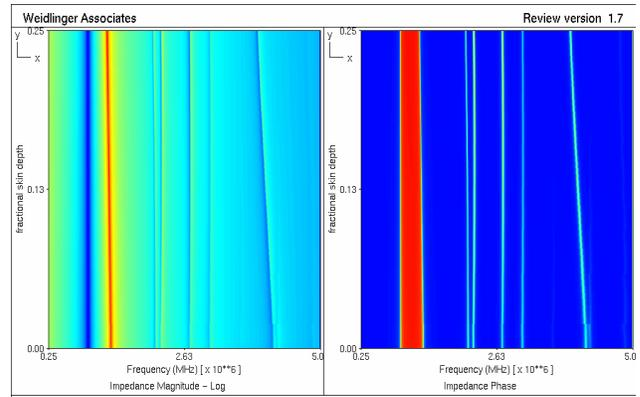
**Figure 14: Impedance response due to skin-depth; 0.75mm wide ( $|Z|$  - left,  $\angle Z$  - right)**
