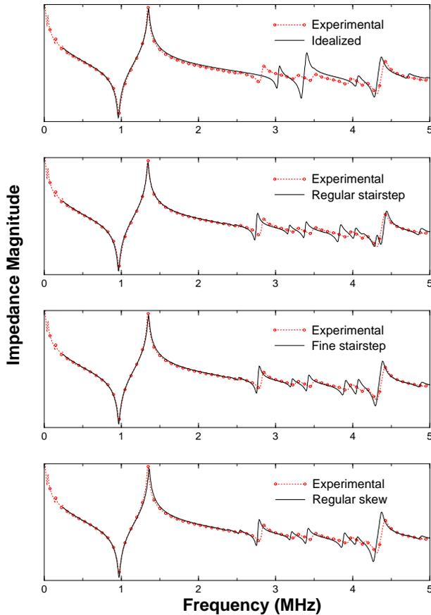
**Figure 6: Impedance response for 0.5mm wide trapezoid**
