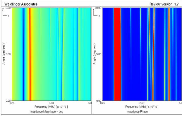
**Figure 11: Impedance response for 0.5mm wide parallelepiped ( $|Z|$  - left,  $\angle Z$  - right)**
