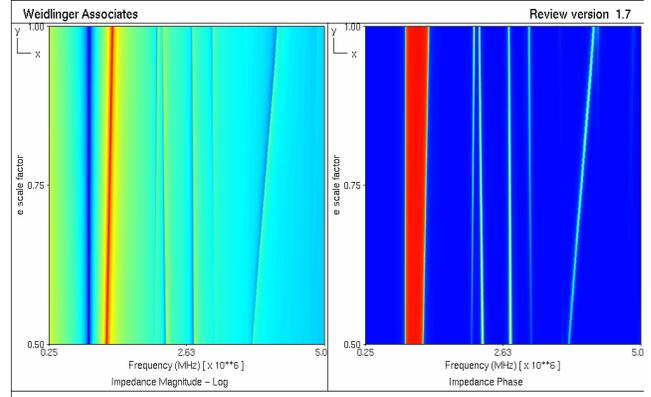
**Figure 13: Impedance response due to depoling; 0.75mm wide ( $|Z|$  - left,  $\angle Z$  - right)**
