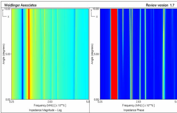
**Figure 12: Impedance response for 0.75mm wide parallelepiped ( $|Z|$  - left,  $\angle Z$  - right)**
