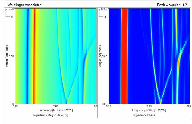
Figure 9: Impedance response for 0.5mm wide trapezoid ( $|Z|$  - left,  $\angle Z$  - right)
