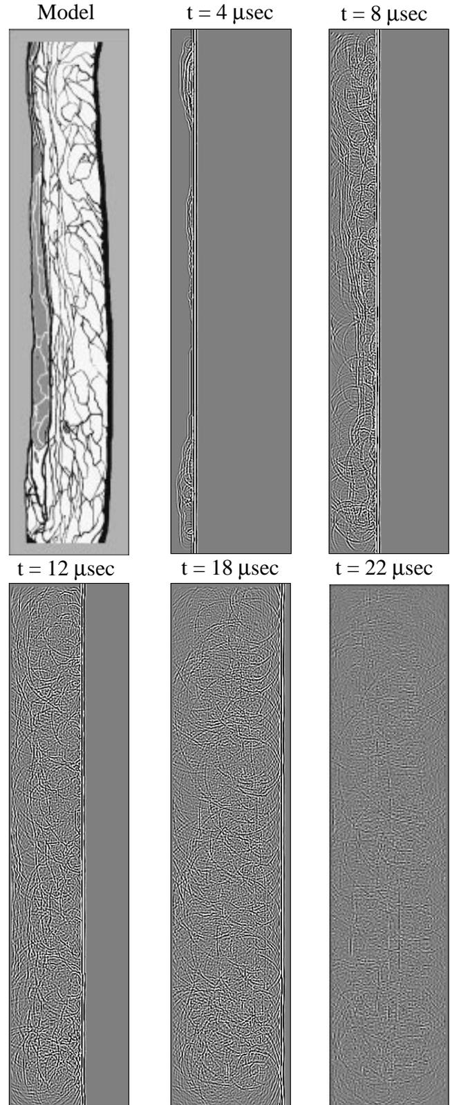
Fig. 5. Large-scale PS calculation of a 2.5 MHz plane wavelet propagating through a 2.1 cm x 11 cm abdominal wall cross-section [1]. Model shown in upper left.
