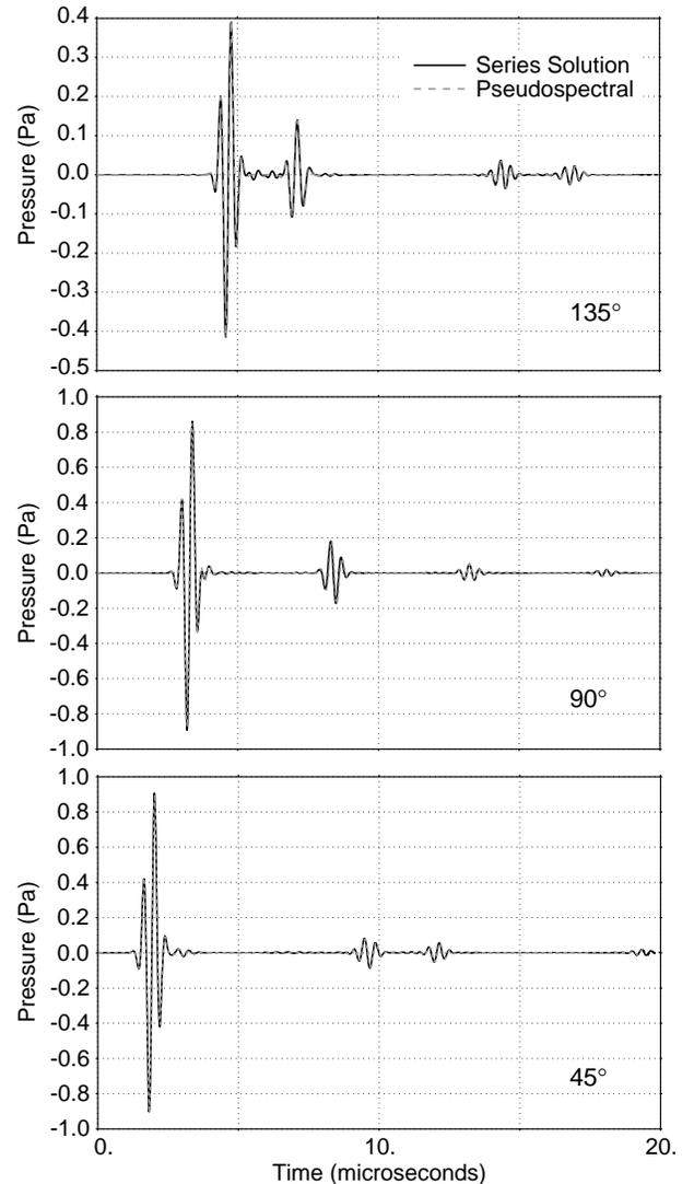
Fig. 4. Validation of the PS method and PML against a truncated series solution at the output points indicated in Fig. 2.
