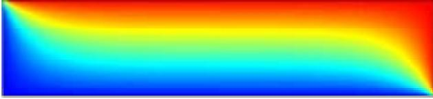
**Figure 4:** Equipotential contours in an element with wraparound electrodes
